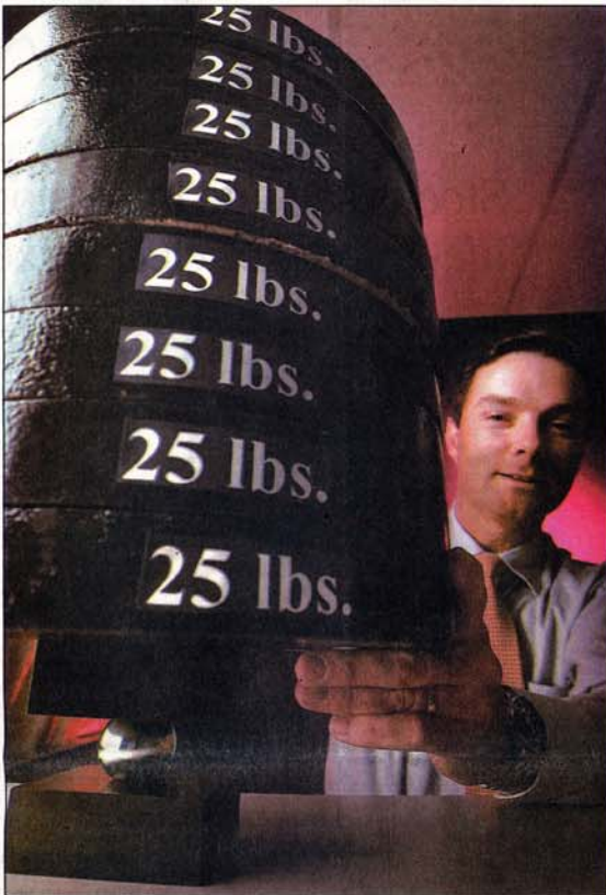
PowerMetal Technologies CEO Edward Hughes, shown here stacking weights on a nanometal-coated pingpong ball, seeks to improve golf equipment through nanotechnology. Howard Lipin / Union-Tribune
